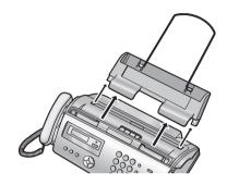
1 Open the front cover (1), push the green button (2), then open the back cover (3).
